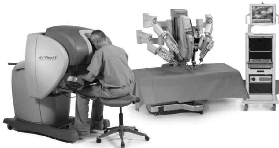
図1 da Vinci® S HD Surgical System (Intuitive Surgical, Inc.) 左 Surgeon console, 中央 Patient Cart, 右 Vision System
